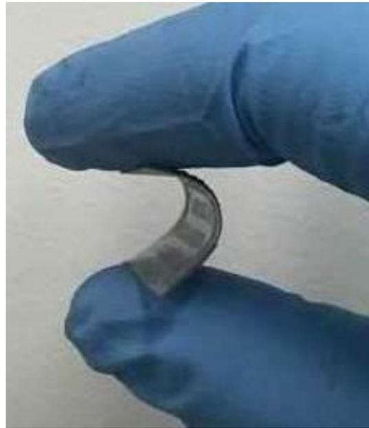
**Figure 7.7** Image of the developed sensor patch depicting its flexibility.
