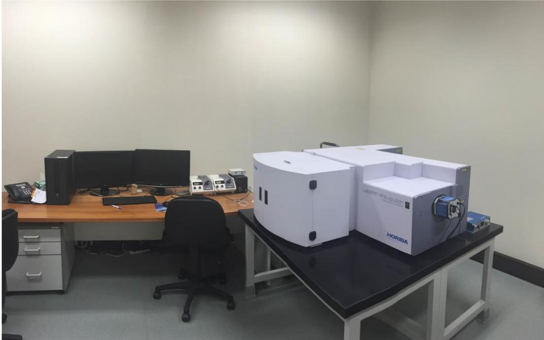
**Figure 2.14: GAU Raman system. Showing (left to right) the computers controlling Raman system, the two light intensity control units, the data recorder and the JY Horiba LABRAM HR Evolution confocal laser Raman system.**
