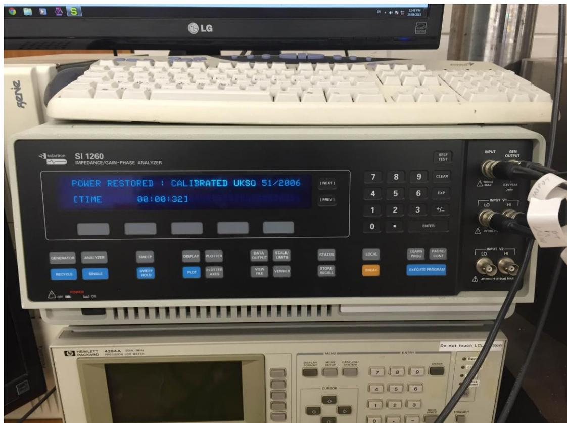
**Figure 2.9:** Solartron 1260A impedance/ Phase-Gain analyser located in the high-pressure laboratory, Macquarie University. During experimentation the four black leads to the right of this image are connected in sets of two (one upper and one lower) to opposing TC wires to measure impedance across the sample. Frequency range, magnitude and time are displayed on the LED screen during measurement.
