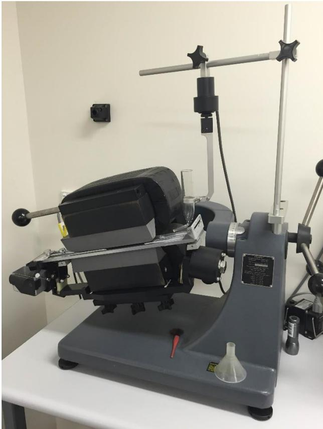
**Figure 2.2: Frantz magnetic separator. Sample is placed in the glass feeder and vibrated slightly to encourage grains to fall. These move past the electromagnets above and below the channel and are separated. Non-magnetic fraction falls to the left with the aid of the 10° side slope. Magnetic fraction is carried along past the centre divider and is dropped into the magnetics catcher.**
