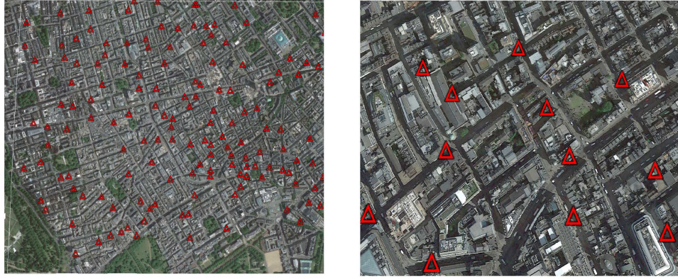
Figure 4.2: Distribution of BSs in the urban region of United Kingdom. Total number of BSs are 161 in the region of 2 \times 1.8 \text{ km}^2 region. Red triangles represent the locations of BSs. (Left:) Overall view. (Right:) Close up view.
