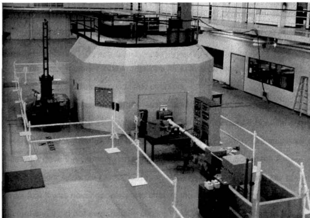
The new reactor Moata, showing the neutron time-of-flight spectrometer installed. The beam tube extends from the reactor face to the beam trap. Associated counting equipment is nearby.
