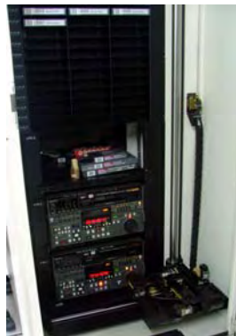
Picture 41: A Mechanical/ Robotic Arm for Inserting Video Tape into the Video Player
