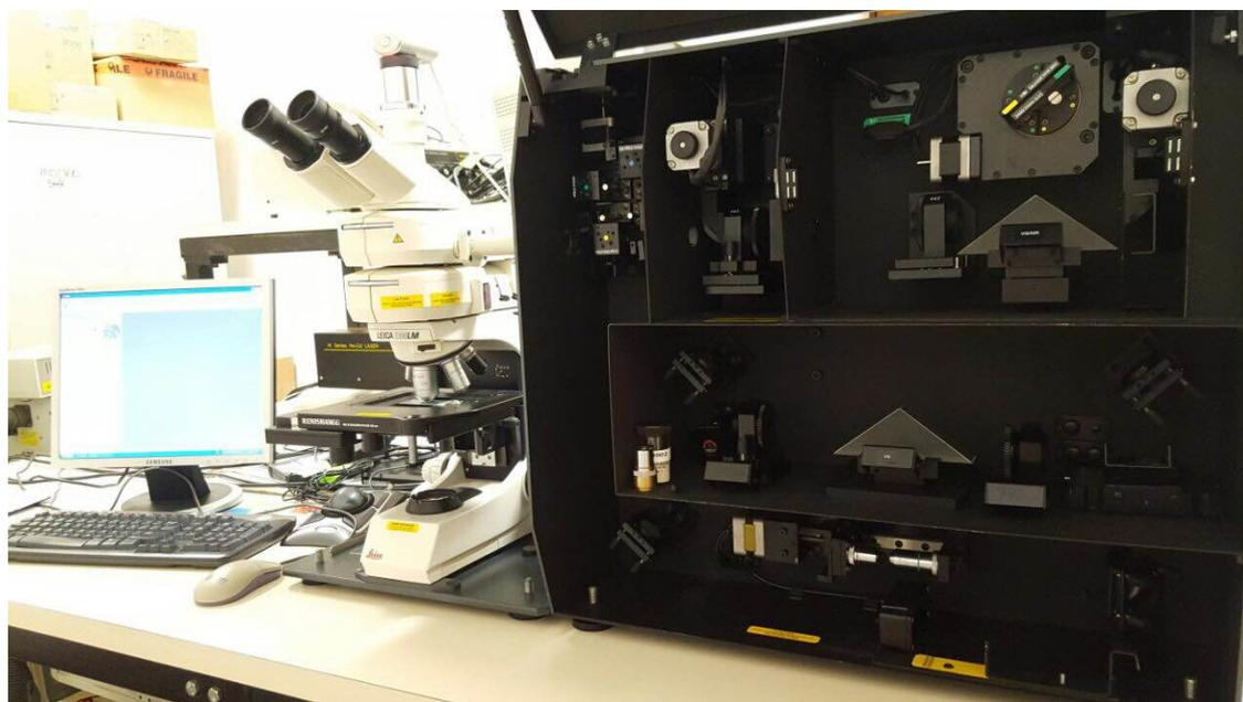
FIGURE A.1: The photograph of our Renishaw InVia Raman spectrometer.
