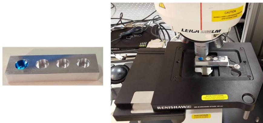
FIGURE 4.10: (a) Aluminium structure designed as sample holder, (b) MB solution in the aluminium structure under the microscope of the Raman spectrometer.
