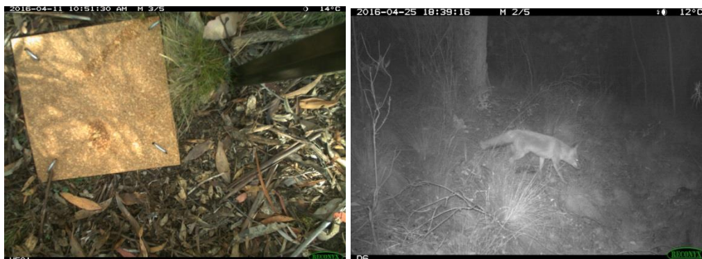
Figure 8. The image on the left was taken by the TYPE WF camera trap and shows the cork tile on which two separate attractants have been placed. The image on the right was taken by the TYPE IR camera trap, designed to detect larger species in this case Vulpes vulpes .
