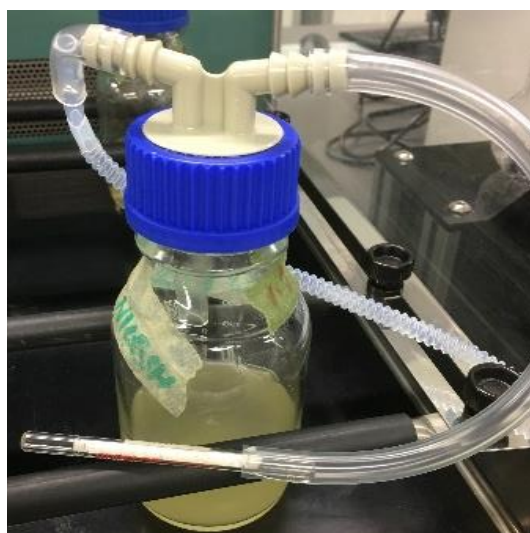
Figure 7: Schott bottle delivery system with TD tube
