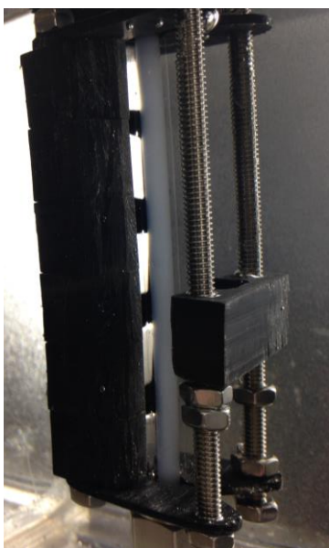
Figure 24: Image showing the constructed 4.0 mm column and modified magnet apparatus.
