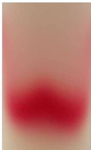
Figure 17: Solute profile of a 50 \mu\text{L} injection of 12 \text{g L}^{-1} iodine CTC solution on a 15 mm ID column 7 minutes into its elution.
