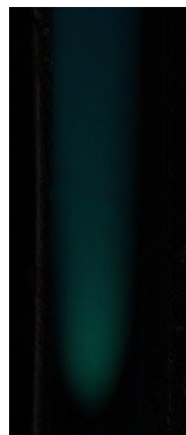
Figure 25: Solute profile of a 10 \mu\text{L} injection of 12 \text{g L}^{-1} iodine in CTC solution on a 4.0 mm ID column 2 minutes into its elution.
