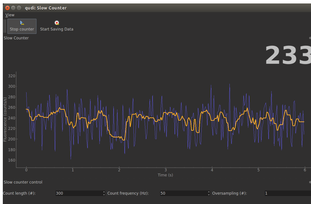
Figure 5.18: Qudi counter GUI for observing the fluorescence signal. The blue curve is the raw data signal as a function of time with a customisable moving average in yellow.
