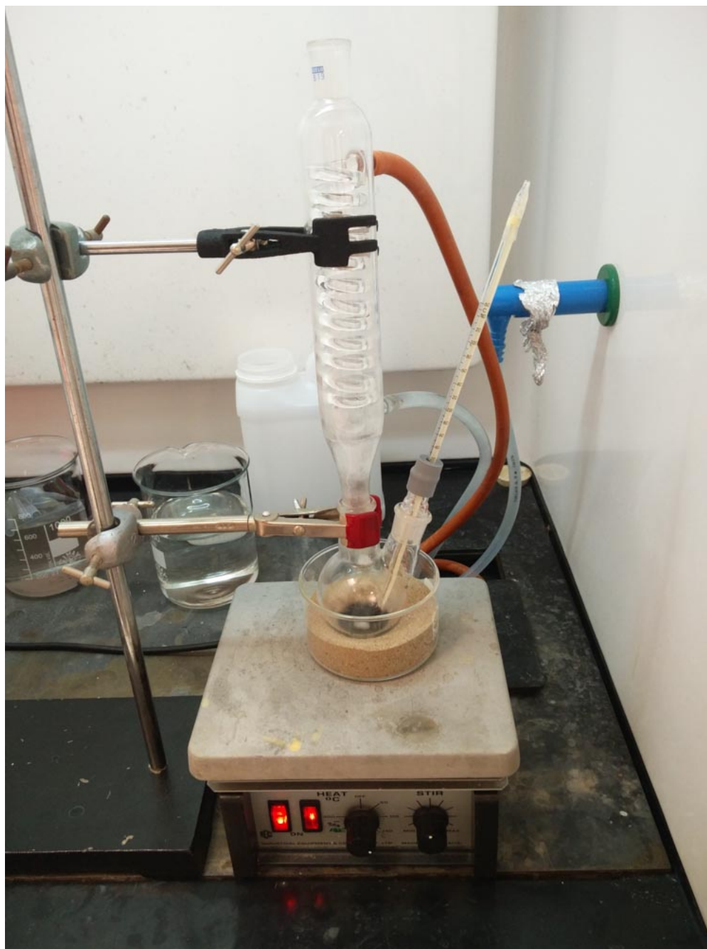
Figure 5.8: Image of the acid boiling treatment process on the nano-diamonds containing many SiV centres to remove the unwanted surface impurities coating the nano-diamond. The solution sits in a round bottom flask in a heated sand bath. A thermometer is placed in the solution to measure the temperature of the acid nano-diamond mix. Above the solution is the water cooled glass condensor to ensure that no nano-diamond material is lost.
