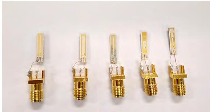
**Figure 4.2:** SMA connectorized eddy current sensors.
