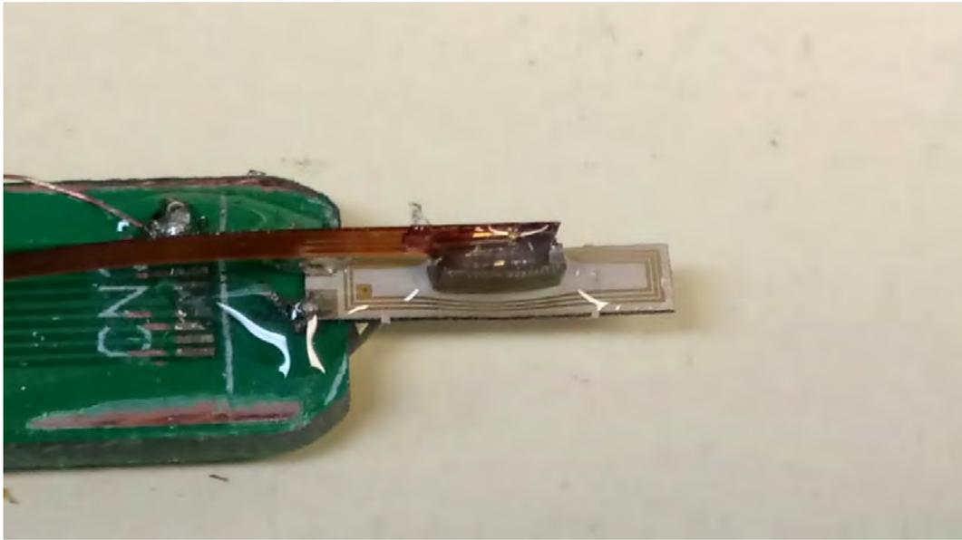
**Figure 4.20:** EC-TMR sensor integration.
