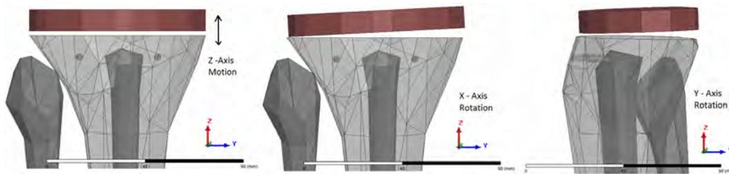
**Figure 2.2:** 3 degrees of freedom of the orthopaedic implant.
