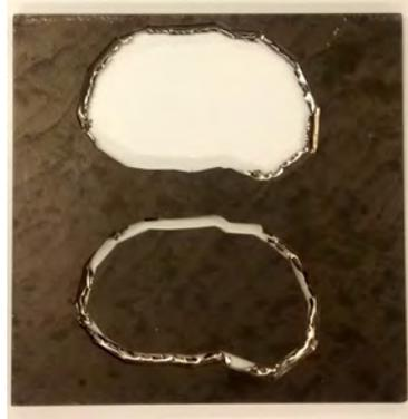
**Figure 4.1:** Tibial implant cut from the titanium sheet of thickness of 4 mm.
