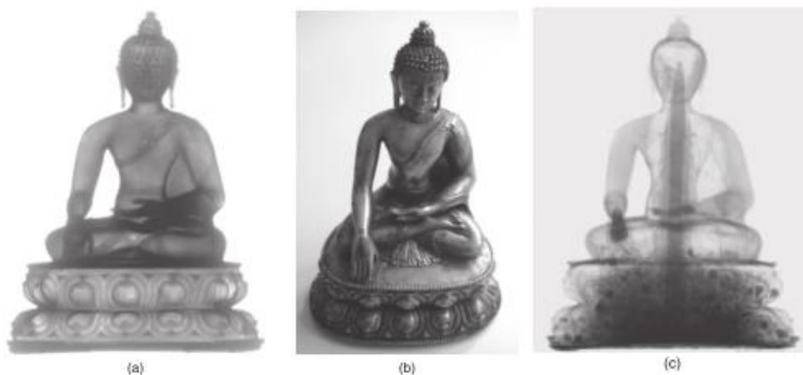
Figure 9. a ) X-ray radiograph of Buddha statue. b ) Photograph of Buddha statue. c ) Neutron tomograph of Buddha statue (Lehmann, Hartmann and Speidel, 2010).
