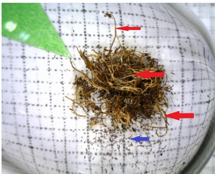
Fur sample ( Beta-473336 ) after pre-treatment; Fur has broken down into smaller particles (blue arrow), and majority of sample is plant material (red arrows).
