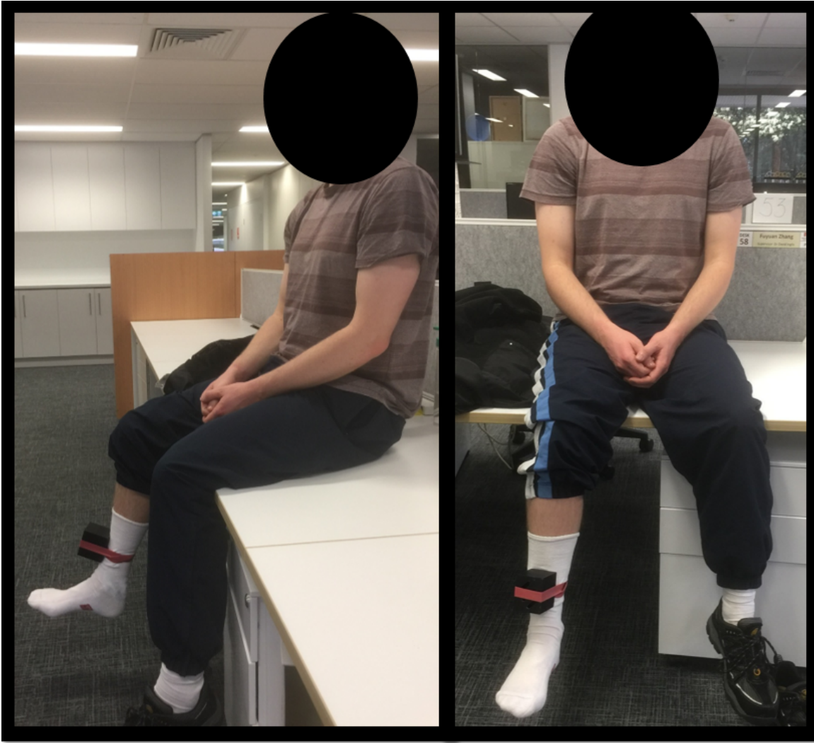
Figure 3.4: Side and front on views of the human experimental setup and WATD placement during the PT. The WATD is secured to the right shank close to the ankle.
