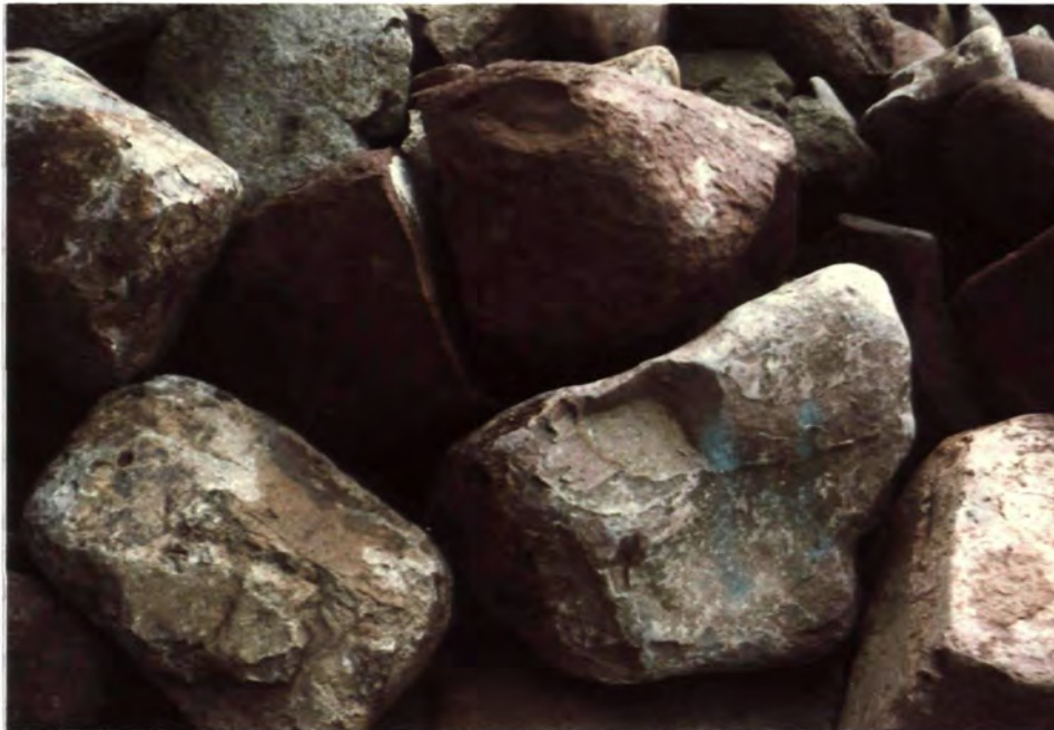
Plate 15. Impact fractured boulder showing shape alteration by breakage. Two sphere shapes have been produced by the splitting of a rod-shaped boulder.
