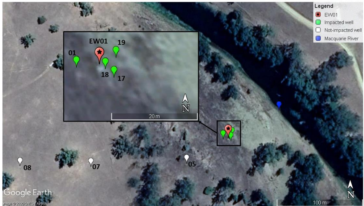
Figure 3. 1: Distribution of monitoring wells, abstraction well and river sample location within the experimental field station at Wellington (NSW) (modified from Google Earth, 2018). Colour legend: red - abstraction well (EW01); green – impacted well; white – Not-impacted well (Control); blue – river sample collection spot.
