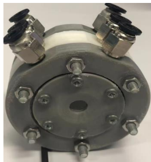
Figure 3.1 Home-made flow cell assembled in a 3-compartment mode.
