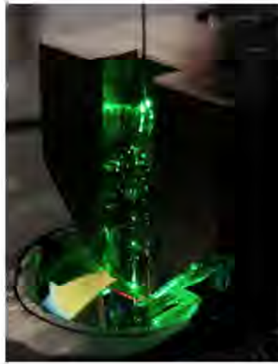
Figure 1.3: A fibre cavity apparatus loaded with an NV rich diamond sample. The green laser at \sim 532 nm is pumped through the cavity fibre. The red emission from the NV centres with the green laser pumping is clearly visible in the picture.
