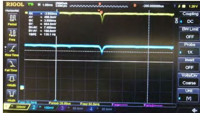
Figure 4-7 the reflected pump signal (yellow and blue) in the scanning mode of the piezo
